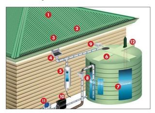
Figure 5 - Illustration of a Rainwater Harvesting System.
