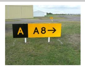
Movement Area Guidance Sign Movement Area Guidance Sign (MAGS) are used to indicate to pilots their position on the airfield. They are also used for drivers to check their position.
