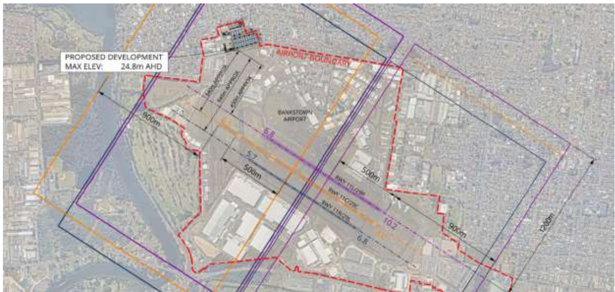
Figure 2 Aerial View of Proposed Development Site Showing Location to the Runway Centreline.
