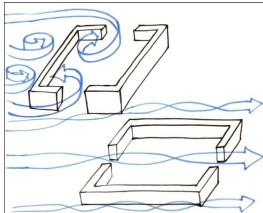
**Figure 8 - Effects of opening placement in relation to wind directions.**
