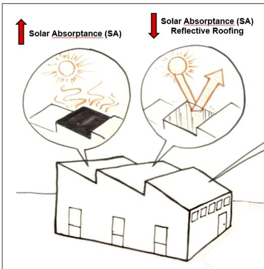
Figure 6 - Effect of roofing solar absorption (SA).
