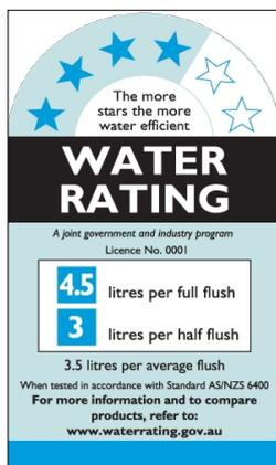
**Figure 4 - Illustration of WELS rating label.**
